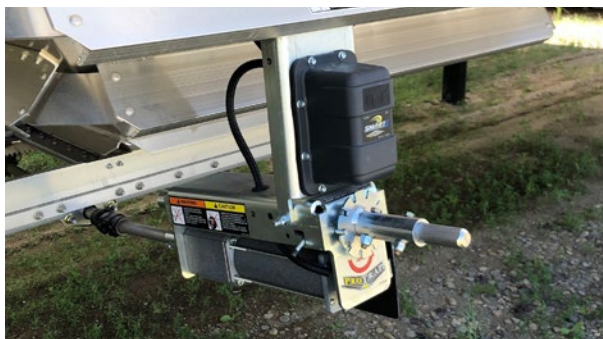
Figure 17 – Shur-Co Electric Chute Gate Drive
