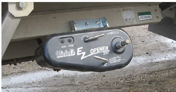
Figure 16 – Michel's Electric Chute Gate Drive
