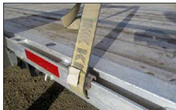
Figure 18 –Flat Hook (Typical)
