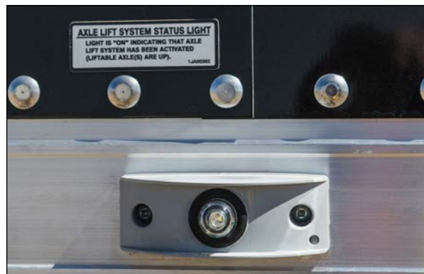
Figure 24 – Axle Lift System Decal and Light
