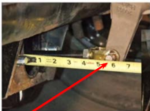
Check released pushrod measurement.
