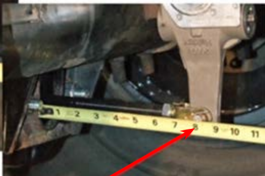
Check applied pushrod measurement at 90–100 psi. Subtract the difference. This is the stroke measurement.
