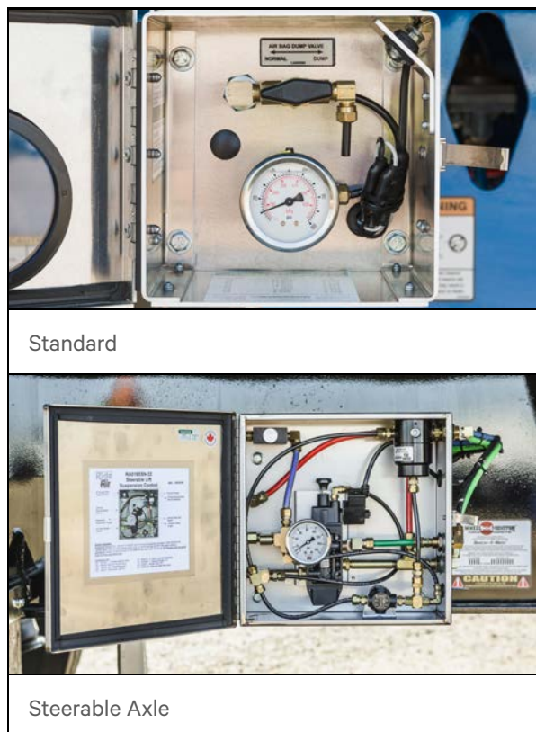
Figure 32 – Air Dump Valve with Gauge
